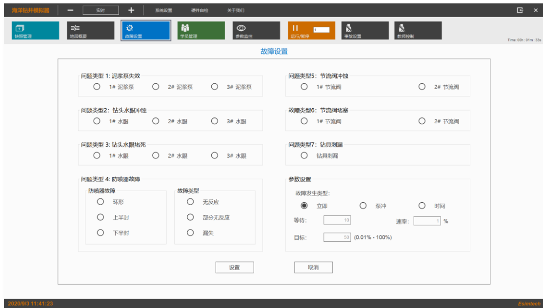
Figure 14 Fault handling software module
