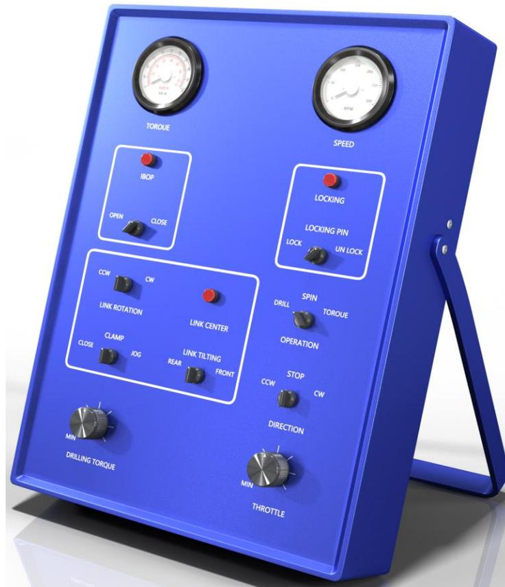
Figure 3 Portable top drive console
